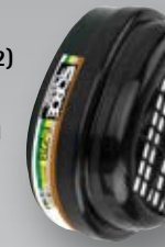
Force™ Classic ABEK1P3 (F-2713) Organic / Inorganic/Acidic Ammonia Vapours and Gases plus Solid and Liquid Particulates
